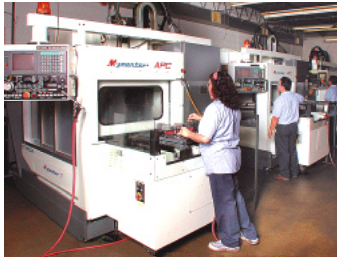
Dynamac currently runs 20 CNCs, 10 of them Kitamura Mycenters. The Sparkchangers (left) use rotary pallet changers, the APCs use pallet shuttles
