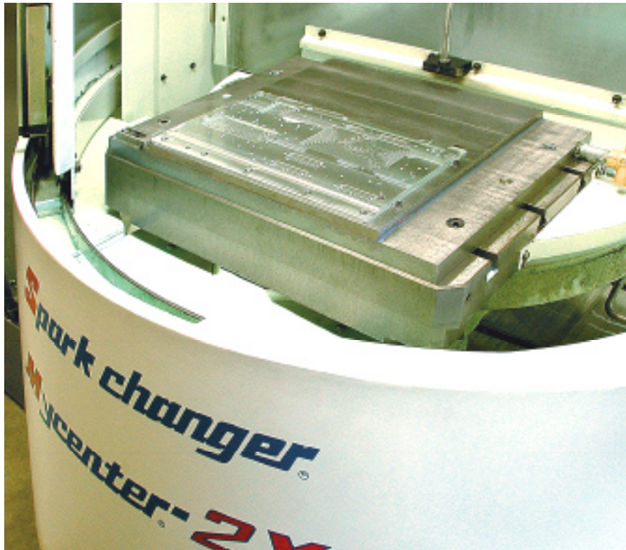
Because conventional clamping distorted the part, Dynamac developed special vacuum fixtures to hold this printed circuit board carrier plate flat during machining. Fixture also avoids interference between clamps and cutters
