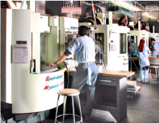
Dynamac currently runs 20 CNCs, 10 of them Kitamura Mycenters. The Sparkchangers (left) use rotary pallet changers, the APCs use pallet shuttles
